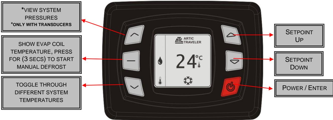
The controller contains a main CPU and is composed of a keyboard for programming and controlling of the refrigeration system, a buzzer for warnings and a screen for viewing parameters, operating status, battery voltage and temperature.
